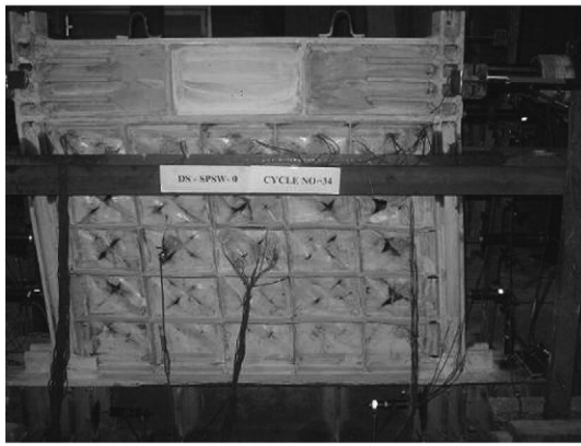
Fig. 5. Deformation of DS-SPSW-0% specimen at 6.44% drift.
